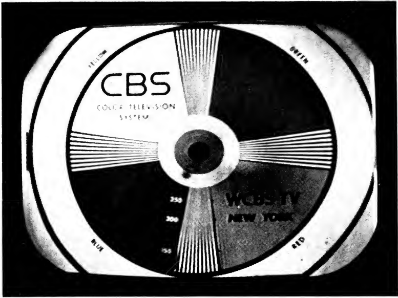
Fig. 10. Test pattern, transmitted with 4.5-mc cutoff frequency, crispened.
